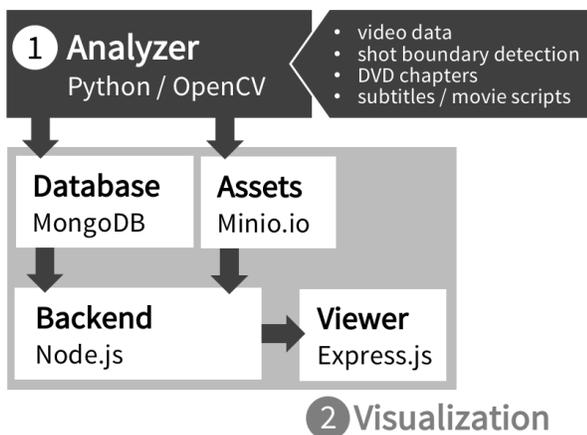
Figure 4: System architecture and components.
